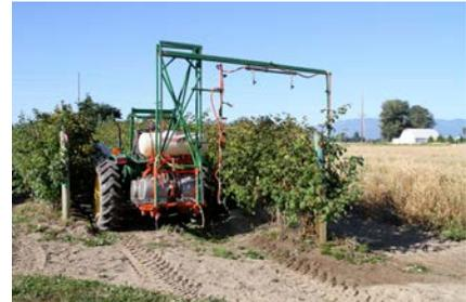
Fig. 1. Over the row boom application of mycoinsecticides to red raspberry hills.
