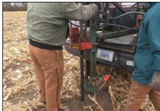
Figure 3. Truck-mounted penetrometer similar to the one to be used in this proposed study.
